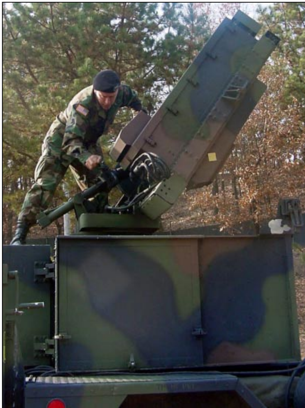
Spc. James Book, HHB 5th Bn. 5th ADA, turns the crank to raise the radar of the Sentinel system. Sentinel crews must fully set up the system in 15 minutes.
