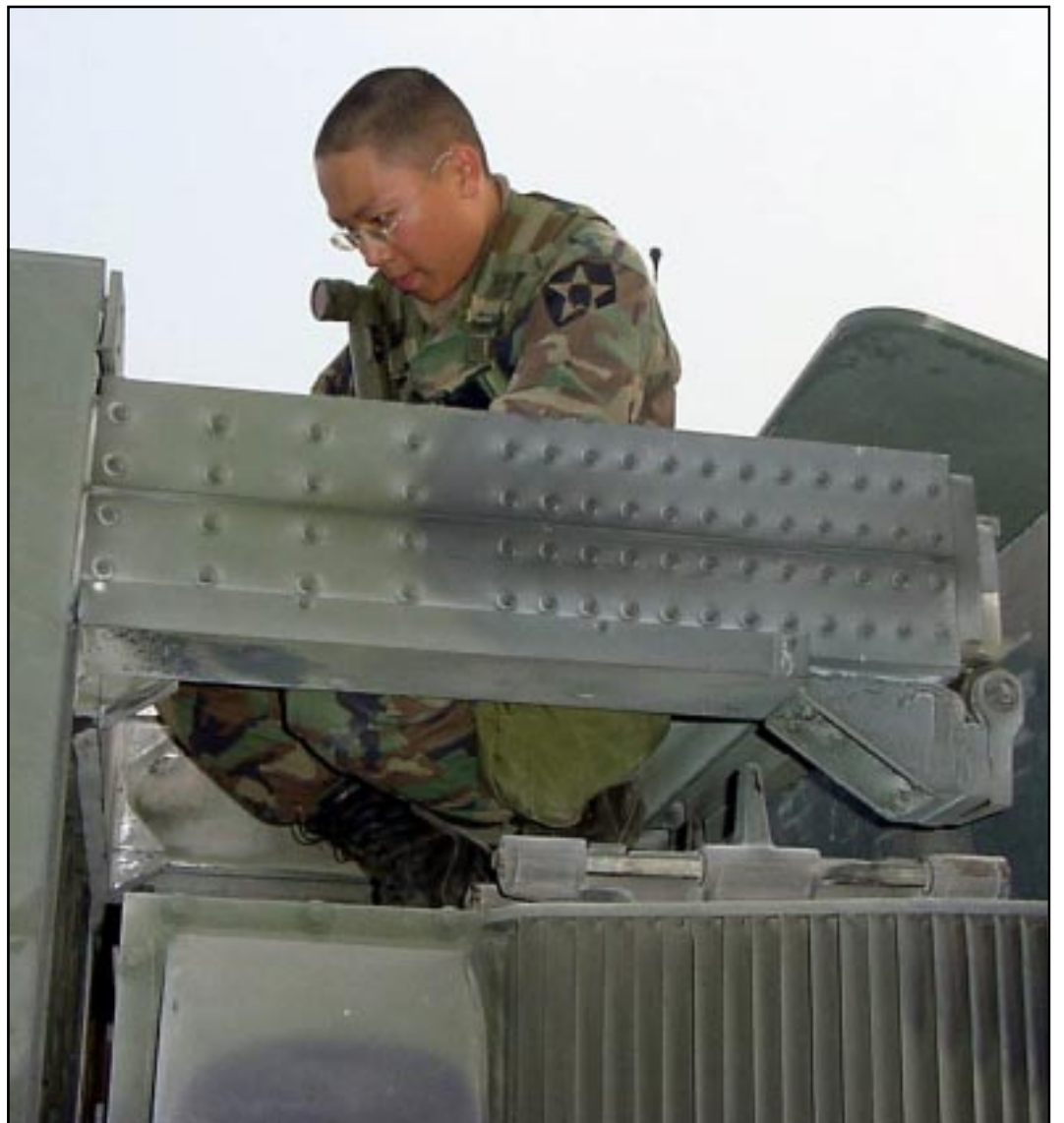
Sgt. Ham, Hyng Kil, 1st Bn. 38th FA, scrapes scorch marks from the MLRS. Rockets fire out from the MLRS with speeds up to twice the speed of sound.
