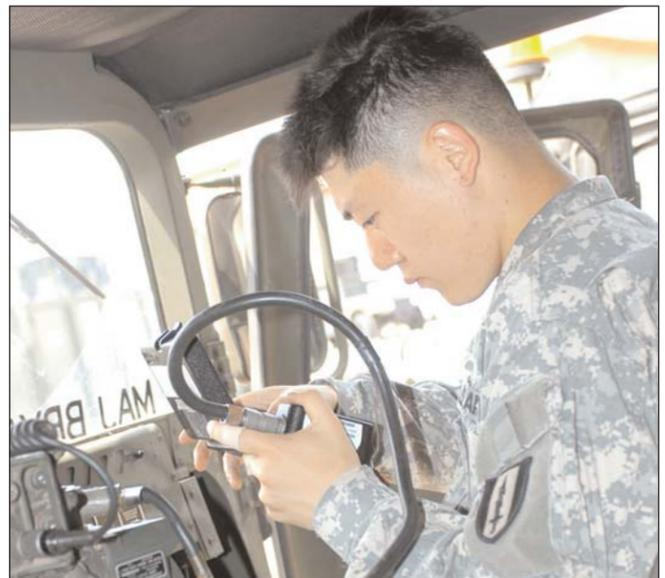
2nd Lt. Paul Lee assembles the radio SINCARS (Single Channel Ground and Airborne Radio System).
