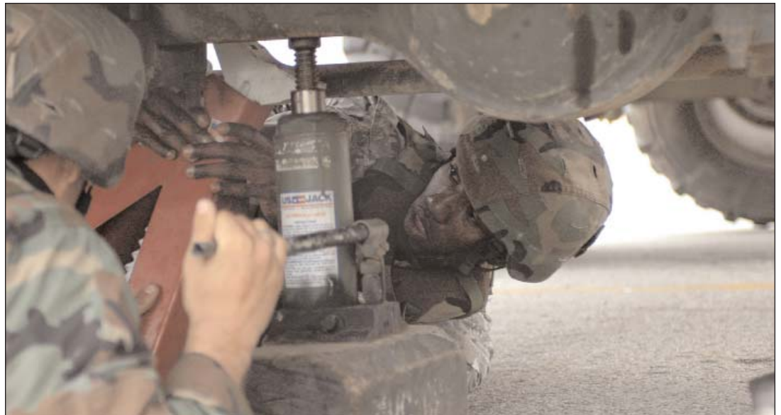
Spc. Iginard Desamours and his teammate place a jack under an LMTV during 302nd BSB's Truck Rodeo competition March 27.
